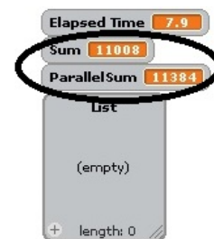
Figure 7: This output shows program variables and the differing sums when the race condition occurs.
