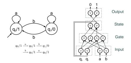
Figure 2. A simple Moore-machine, the processing of the input word *abba* (left) and a corresponding McCulloch-Pitts-network (right).
