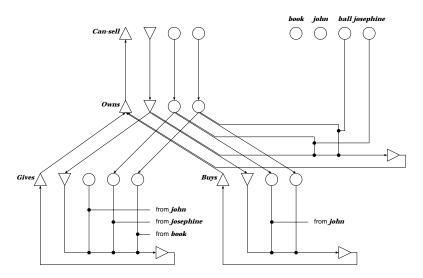
Figure 4. A SHRUTI network for the knowledge base from Table 2. Each predicate is represented by two *relais units*  $(\triangle, \bigtriangledown)$  and a set of *argument units*  $(\bigcirc)$ . Constants are represented as  $\bigcirc$ -units in the upper right. Facts are implemented using  $\triangleright$ -units.
